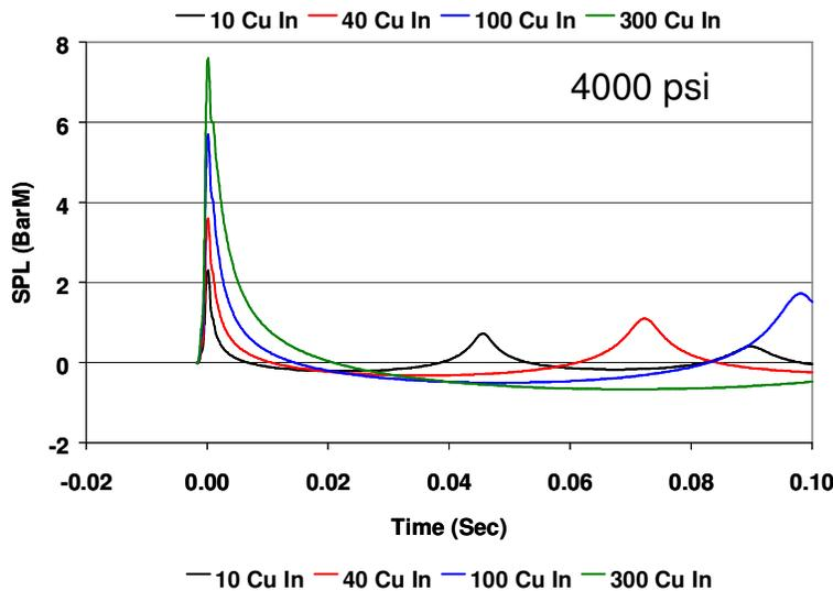
These plots show the acoustic signal generated by air guns with different chamber volumes for supply pressures of 2,000 and 4,000 psi. The peak pressure generated by an air gun increases as the volume of compressed gas is increased – going from near three BarM with the 10 cubic inch chamber suggested for pinniped control, to nearly eight BarM for the 300 cubic inch chamber.
