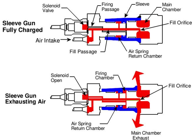
opens the sleeve or poppet valve, and releases the high pressure air into the water. The air spring return chamber and the reducing pressure in the main chamber allow the sleeve or poppet valve to close and the main chamber to recharge to the high system pressure. The high pressure air that was released into the water expands rapidly and then oscillates like a spherical bubble until all of the energy is dissipated (typically in less than 0.1 seconds). The
